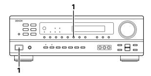
When the main unit's power operation switch turn on while pressing the set's MEMORY button the unit automatically begins searching for FM broadcast stations.
